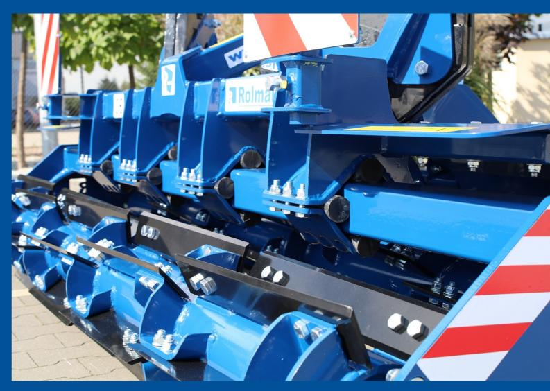
The ProCut front knife roller works perfectly in the field, as a solo device, as well as in combination with other tillage machines mounted on the tractor's rear jack. The ProCut knife roller at the front and the disc harrow operating at the rear of the tractor constitute a perfect combination and they are a recommended set of tillage cultivators for stand after corn.
