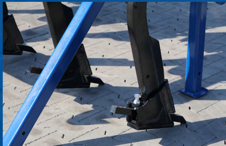
ATLAS tine set to operate as a subsoiler
