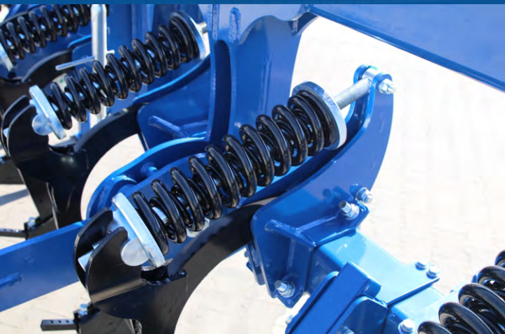
Double spring of the non-stop protection
